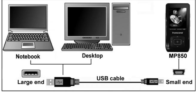
Figure 4: Connecting to a Computer
